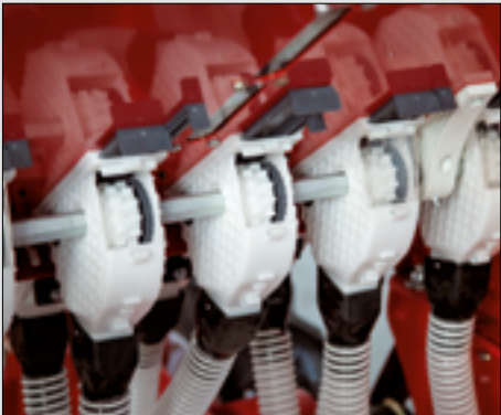
Seed distributors for seeding small, medium and large seeds 播种小型、中型和大型种子的种子分配器
