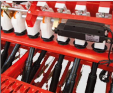
Electric or solenoid (optional) valves for tramline control 电动或电磁(可选)阀门行关闭系统
